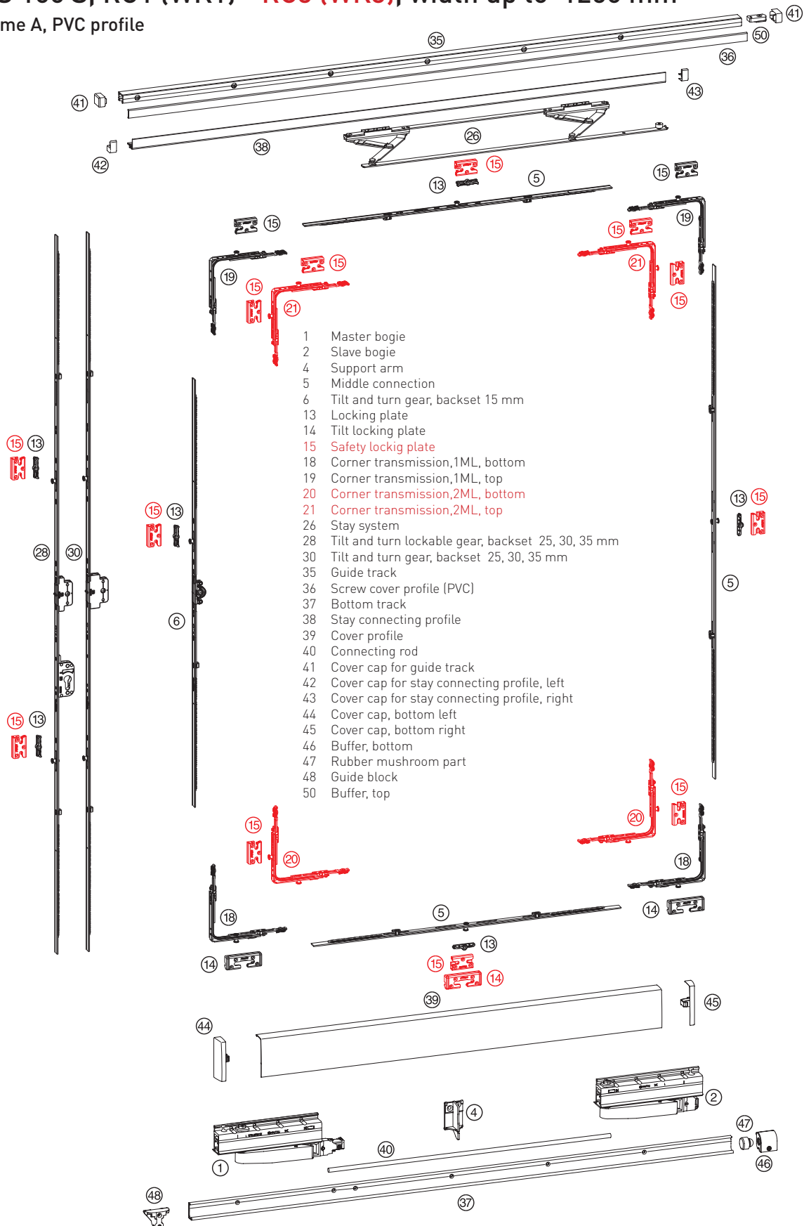
Figure fitting parts = design left (according to DIN EN 12519 opening to the right)
