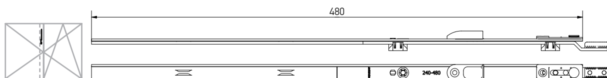
Extension lock, double sash 480 mm
