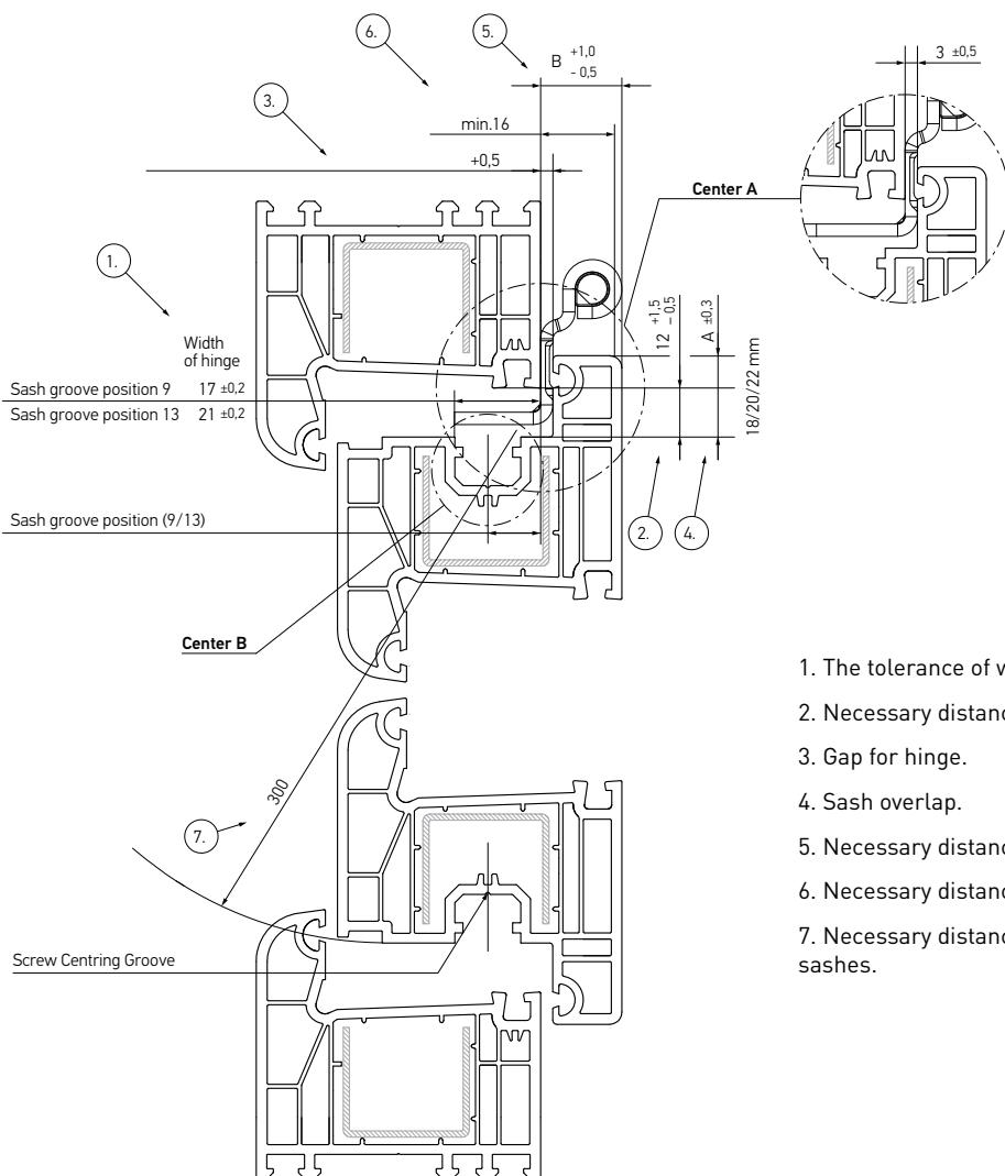
1. The tolerance of width for top sash's hinge.
